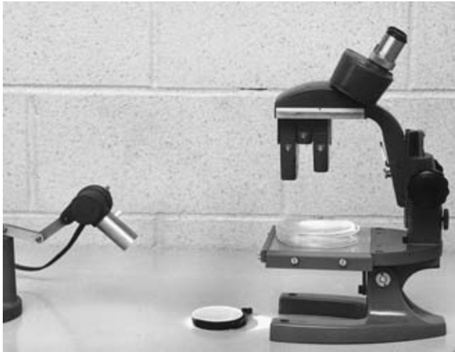
19.4. Arrangement of stereomicroscope with obliquely transmitted light for evaluation of colonial morphology.
