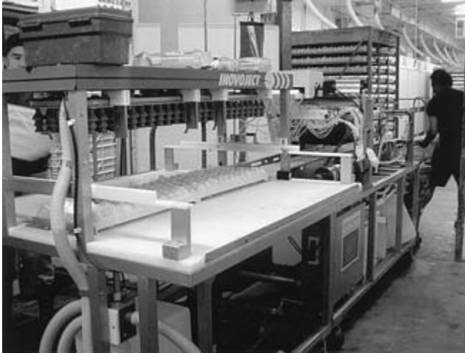
Fig. 1.8. A modern hatchery with an egg injection system for in ovo vaccination.
